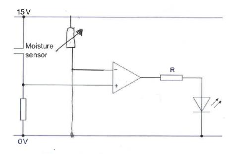
The comparator has saturation values of 14 V and 0 V.
