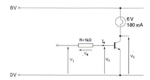
(a) The input voltage V<sub>1</sub> = 0.2 V. Complete the table below. The transistor is switched off.
