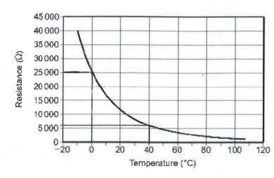
(a) State the resistance of the thermistor at 0 °C. 25 K-SZ
